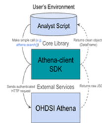
Figure 1: Depicts how the SDK mediates between the user and Athena endpoint
